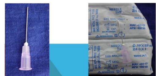
Fig. 2: To see the size 24 No. hypodermic needle (0.56 mm in diameter) was used
