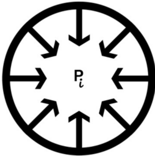
Fig. 1: The inward recoil tendency of the elastic wall is counterbalanced by the development of excess pressure force in the fluid. At equilibrium, the tendency of the contents to recoil outwards is equal to the tendency of the wall to contract or recoil inwards
