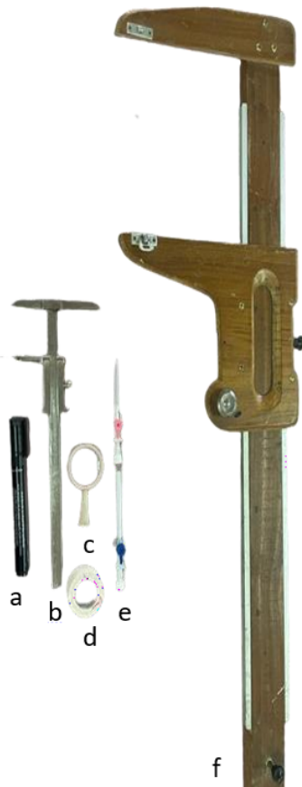
Figure 1: Instruments; (a) Marker pen (b) Vernier caliper (c) Handles (d) Adhesive tape (e) Hypodermic needle (f) Osteometric board
