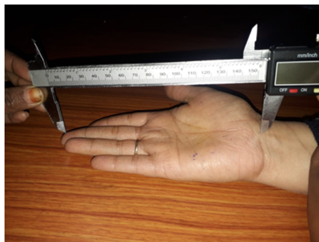
Fig. 1: Measurement of hand length using a digital vernier caliper
