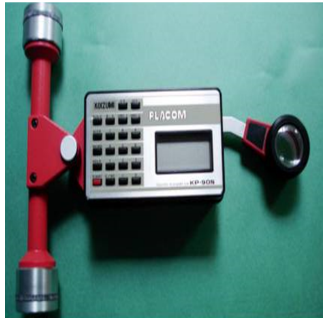
Fig. 4: Showing digital planimeter KP-90N Placom (Lawrence and Mayo (India) pvt. Ltd. 274, Dr. D.N. Road, Mumbai -400001)
